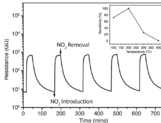
Changes in the resistance of nanoparticulate WO<sub>3</sub> films exposed to 0 and 10 ppm NO<sub>2</sub> in air at 200°C. Inset: Normalized sensitivity of the nanoparticulate films as a function of temperature.
