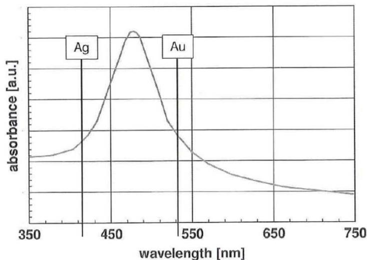
Absorption spectrum of a Au-Ag alloy, ratio 1:1.
