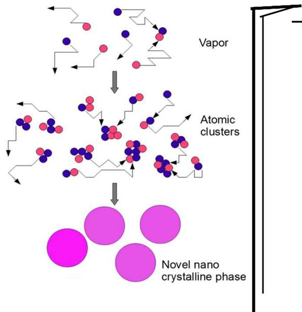
The sparks have to be short enough to produce atomically mixed particles
