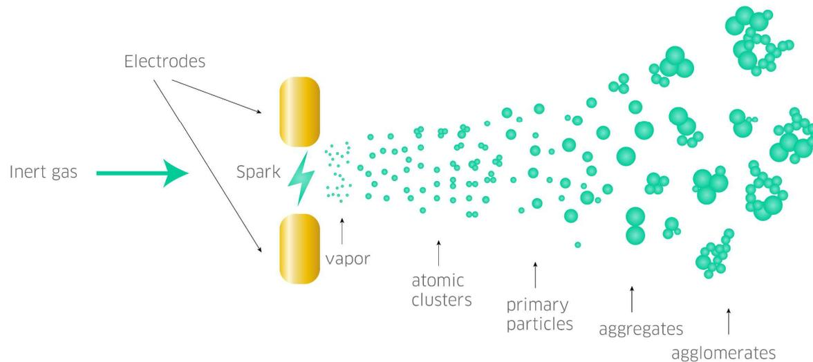
Short (1 – 10  $\mu\text{s}$ ) repetitive sparks produce strongly quenched vapor ( $\approx 10^7 \text{ K s}^{-1}$ )
