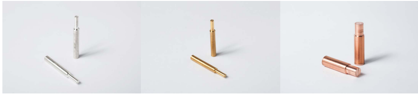
Electrodes (source of nanoparticle production) of different materials
